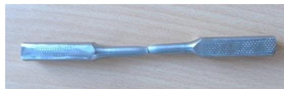
Fig. 3.8 Tested tensile specimen after the test.
